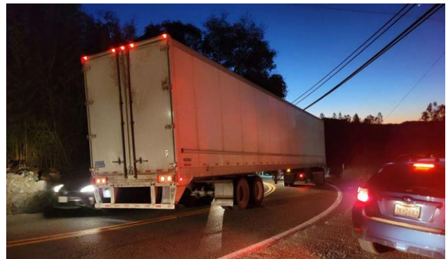
FIGURE 2: OVERSIZE TRUCK TRACKING INTO OPPOSITE LANE
